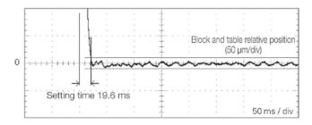
(c) Model following damping control and feed-forward damping control
