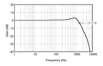
Fig 3: Frequency response curve
