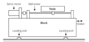
Fig. 4: Movable unit mounted atop a block
