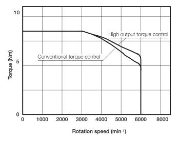
Fig. 2: Torque vs. rotation speed characteristics
